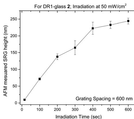
Fig. 7 SRG height as a function of irradiation time for DR1-glass 2.
