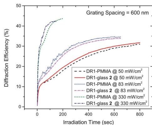
Fig. 6 Diffraction efficiency as a function of irradiation time for DR1-PMMA and DR1-glass 2 at various laser irradiances.
