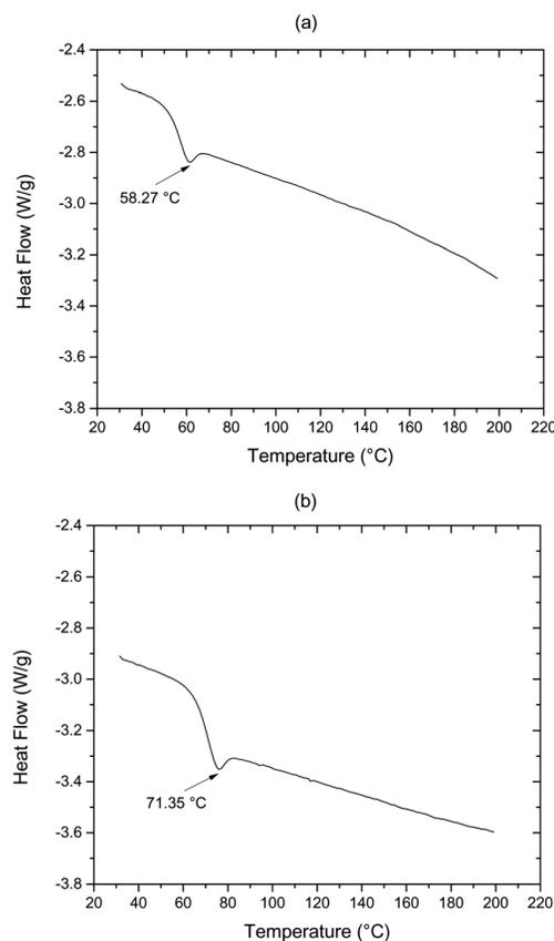
Fig. 1 Representative differential scanning calorimetry scans of (a) compound **1**, and (b) DR1-substituted glass **2**. The scans were recorded at a heating rate of 5 °C min<sup>-1</sup>.  $T_g$  values are indicated. Note the absence of crystallization in both cases.
