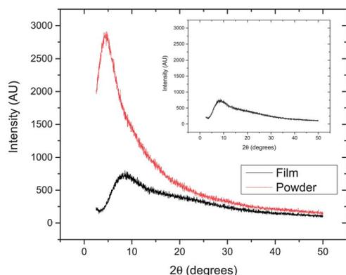
Fig. 3 Powder X-ray Diffraction (PXRD) pattern of a film and a powder sample of DR1-glass 2. The diffraction pattern of the substrate is shown for comparison.
