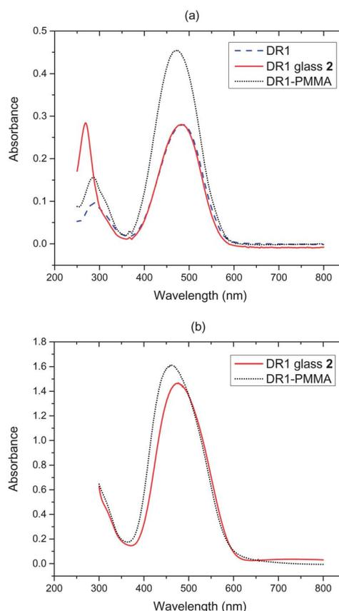
Fig. 2 Absorbance spectra: (a) Disperse Red 1, DR1-glass **2**, and DR1-PMMA in CH<sub>2</sub>Cl<sub>2</sub> solution; and (b) thin solid films of DR1-glass **2** and DR1-PMMA. The spectra in CH<sub>2</sub>Cl<sub>2</sub> solution were recorded using concentrations of 0.01 mM for DR1 and compound **2**, and 0.0006 wt% for DR1-PMMA.
