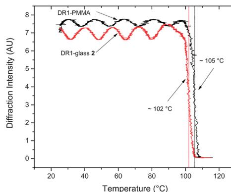
Fig. 8 Diffraction intensity as a function of temperature for DR1-PMMA and DR1-glass 2.
