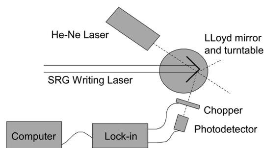
Fig. 5 Experimental set-up for monitoring diffraction efficiency.
